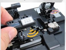
RFID tag equipped to the fiber holder communicate with CT110/CT111 and choose proper cleaving program(\*1)
